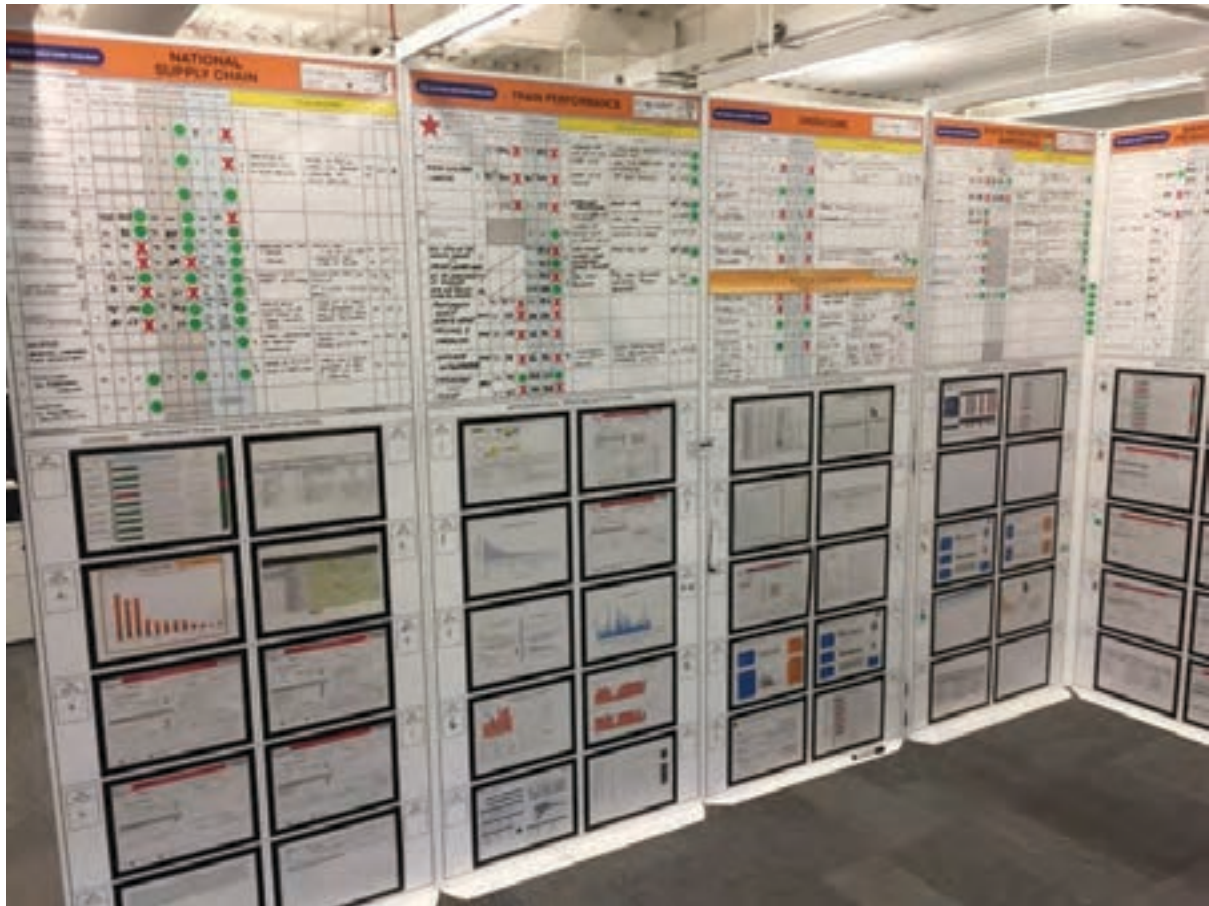
Figure 42. The work boards contain a task tracing section on the left, a problem solving section on the right with the concerns and actions columns and a team performance/KPIs section at the bottom.
