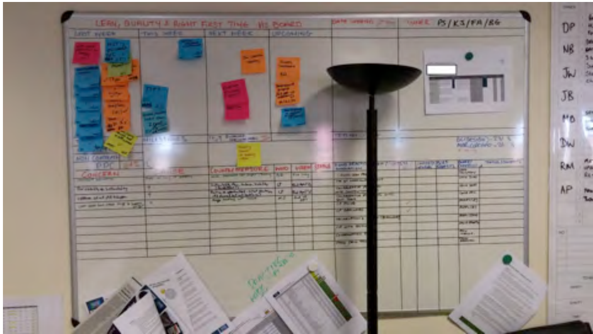
Figure 35. Another Type II CI cell board from Scheme 1. The task tracking section is at the top with colour-coded post-its and the 3C section at the bottom. Although there are many concerns and countermeasures already filled in in the 3C section, many question marks (“?”) were put in the causes column suggesting a hardship in identifying the root cause of concerns.
